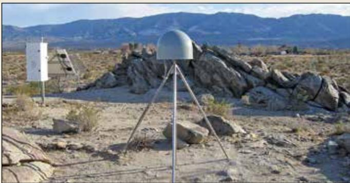
Continuous GPS (CGPS) site (P582) is one of 13 sites in the study area that collected position data in 2016 and can be used to evaluate subsidence. Daily data from a CGPS site and spatially detailed data from InSAR can be leveraged to improve the understanding of compaction processes in time and space. Photograph courtesy of University NAVSTAR Consortium (UNAVCO), copyright 2006 UNAVCO, Inc. (used with permission).
